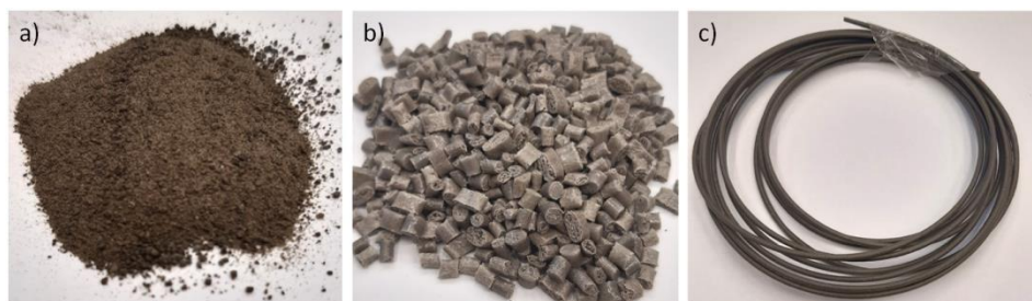
Fig. 1. Steps in the manufacture of regolith-filled filament: a) drying of regolith, b) manufacture of pellets, c) extrusion of finished filament
