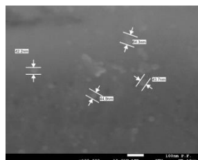
Fig. 1. The microstructures of the coatings on the Armco iron samples after the ESA process, the Mo- SPM -Mo coating obtained at W_p = 0.52 J, the – SPM is the multi-walled ARKEMA carbon nanotubes (0.2%) in the epoxy resin of Epoxy 510 type without a curing agent: at the magnification of: a – 50,000 times, b – 100,000 times
